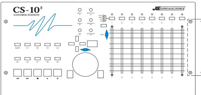
Note that the thin plate slips into the gap between the top cover and the chassis, and cannot be seen. It is *not* mounted on top of the control station.
